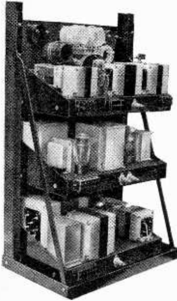
Odeon 50-watt output transmitter covering the 3.5- to 28-Mc/s bands and including modulator and power supplies.
