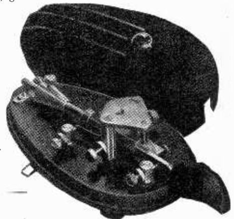
Eddystone automatic key; this type is usually described as a bug-key.
